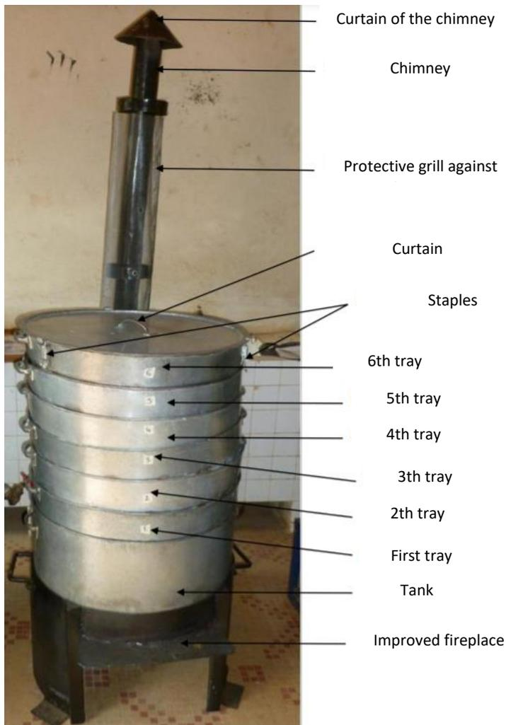
**Figure 1:** Different components of the CUVE ABLO (source : Houssou et al, 2015)
