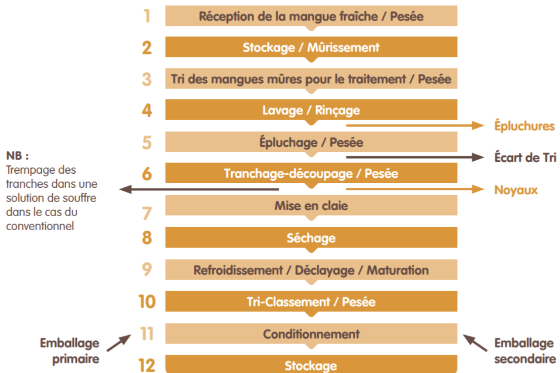
Figure 1 : drying process of the mango (PAFASP, 2017)
